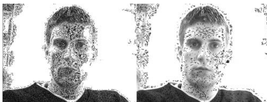
Figure 8: Motion compensated images. Lucas and Kanade (left) and Horn and Schunck (right).
